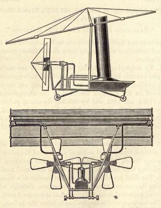
An aëroplane, composed of tubes covered with fabric, is pivotted to the main frame in such a manner that it may be adjusted, up or down, to any required angle.
